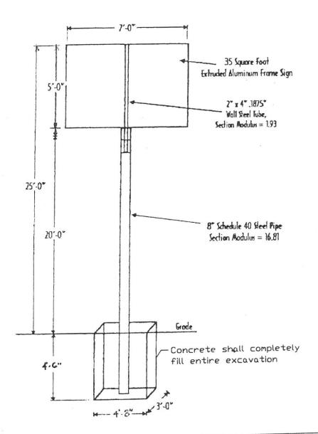
Min. concrete: 3000 psi. Min. soil bearing: 2000 psf.
